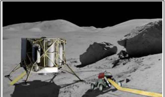
Figure 2. Surface teleoperation of rovers from orbiting facilities is a key technology for astronaut-assisted deployment of a lunar far side polyimide antenna and collection of geological samples. Image is courtesy of Robert MacDowell and NASA GSFC.
